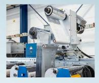
A sturdy top rail makes mounting and moving press assemblies extremely easy.
