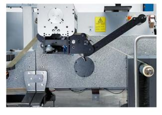
Thanks to its granite core, the press has a particularly long service life and is quieter than any other machine in this class.
