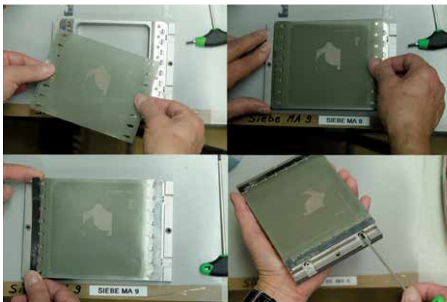
The Screeny G-Line principle: minimal handling to mount the imaging screen printing plates in the frame
