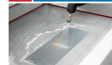
After imaging, the screen printing plate is washed out on both sides with high pressured water and dried on a coarse polyester screen that is clamped in place. After drying, the photo emulsion has an Rz value (surface roughness value) of **less than 5 microns.**
