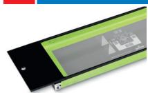
Before printing, the frame's outside and inside edges are masked with silver adhesive tape. A screen printing plate can be changed in **less than 1 minute.**The screen printing plate can be stored quickly and easily in a film folder for repeat orders.
