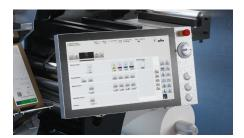
Human Machine Interface (HMI) is designed to summarize important information at a glance. For quality assurance, the print results can be checked live, via web video, or while the press is running.
