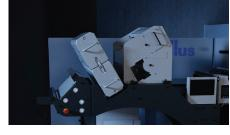
Automatic Splice Detection on the Gallus One automatically detect splices, letting them pass all print bars without loss of register and speed. This results in minimized waste and increased uptime.
