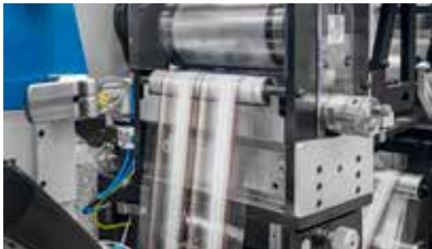
Semi-rotary die-cutting unit with compensator.
