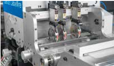
Optional slitter available in rotary blade or razor blade design.
