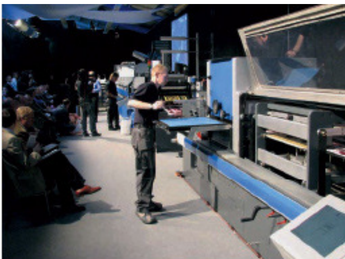
KM 510 S in the Gallus demonstration centre: 8 printing unit press equipped with a screen printing unit and a hot foiling station for the demonstration. The first job was a five colour piece of cosmetics packaging, screen-printed glitter ink and hot-foiled silver which was then creased and die-cut by the inline flatbed die-cutter (picture).
