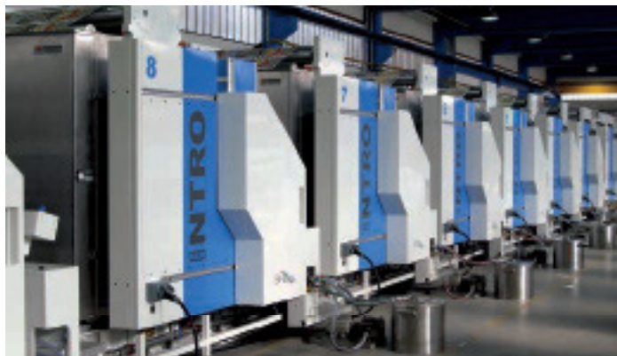
The 9 colour BHS Intro L AFL 1259 press with a web width of 1,295 mm configured for printing with water-based inks and UV coating.
