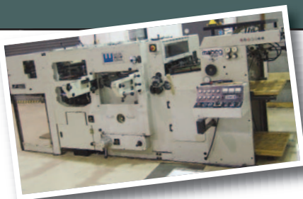
The Iijima die cutter uses the Wupa system of moving lower platen.
