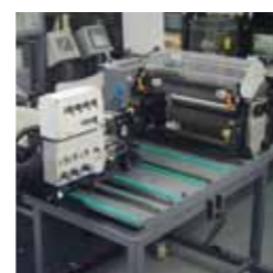
Flexible combination of printing, processing and finishing over the entire length of the machine – can be changed in minutes without tools.
