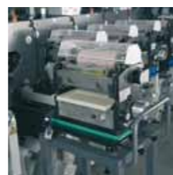
The quick-change platform makes it easy to change between printing units.
