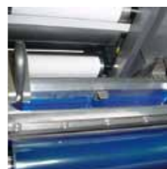
High print speeds thanks to the chambered doctor blade.
