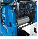
The Gallus Rotascreen rotary screen printing unit for thick ink layers or effective picture features.
