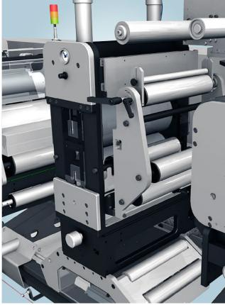
No format-dependent die cutting assemblies thanks to semi-rotary die cutter.
