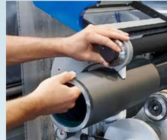
Frontloading anilox sleeve permits quick and easy exchange.
