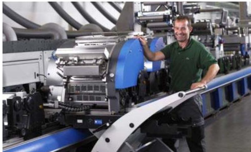
Fig. 1: The flexibility of a press is a key factor for its cost-effectiveness in label printing. The printing units of the Gallus RCS can accommodate any major printing process. The changeover process – shown here on an offset printing unit – takes only a few minutes.
