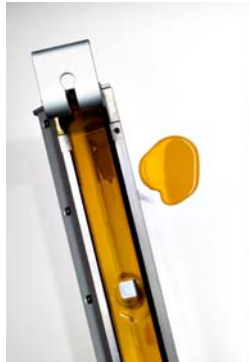
Fig. 4: Chambered doctor blade system on the Gallus ECS 340 ensures fast ink changes
