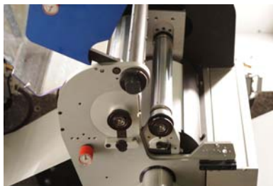
Fig. 6: Extremely short web travel of just 1.1 metres between printing units
